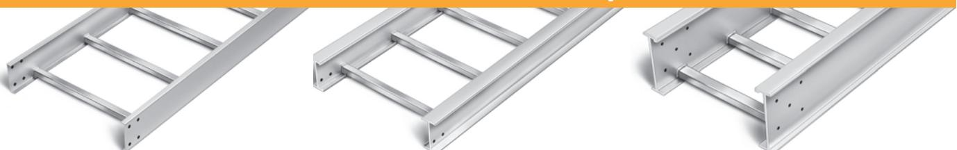
Aluminum cable tray is the most popular tray in use today. Chalfant has a wide offering in aluminum tray from light duty commercial/institutional systems for data and telephone support to utility/industrial grade tray and extra heavy duty long span tray to 30' spans. Ideal for most corrosive atmospheres including offshore, seacoast and petro-chemical applications. Not recommended for use in chlorine, caustic or high acid environments.
