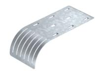
The cable exit plate allows compliance with specific bend radii (fibre-optic cables), thus preventing possible cable breaks. Can be mounted in a lengthwise direction and at the side, can be arranged for greater widths.
