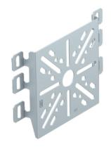
Mounting plate, for fastening on the side rail of cable support systems. Please order the truss-head bolt, type FRSB 6 x 12, separately.
