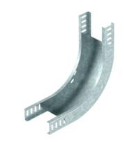
$90^{\circ}$  rising vertical bend, for all cable tray types of 35 mm side height. The vertical bend is pushed over the end of the cable tray and screwed tight. Fastening materials should be ordered separately.
