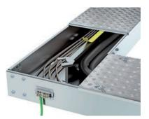
Equipotential Bonding Walkable cable tray systems shown with equipotential bonding rail installed.
