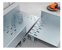
Creating changes of direction 90 ° For this, the cable trays with the appropriate tools and machines are so cut that this blunt lie to each other. After nesting of cut cable trays they are screwed together by means of longitudinal angled connectors.
