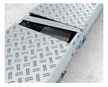
Using the dust protection element The dust protection element type SSE is there to prevent the intrusion of foreign particles such as sweat, dust or similar at the butt joints of the covers. The dust protection element is simply pushed between steel sheet and aluminium sheet of the first cover and is therefore easily held in position.
